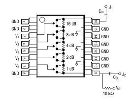
DC blocking capacitors (C\_{BL}) and biasing resistor must be supplied externally for positive voltage operation. C\_{BL} = 47 pF for operation >500 MHz.
