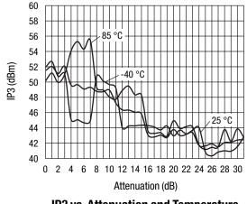
IP3 vs. Attenuation and Temperature
